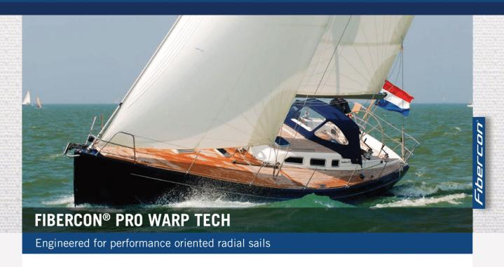
Contender's Fibercon® Pro Warp Tech range is the latest addition to the Contender line of woven polyester sailcloth for radial applications. With a special weaving technology Warp Tech constructions feature a combination of uncrimped heavy warp yarns for low load elongation with finer denier warp and fill yarns creating a tight and balanced weave. This makes Warp Tech unique as it provides very low warp stretch without compromising good bias stability and fill strength.
